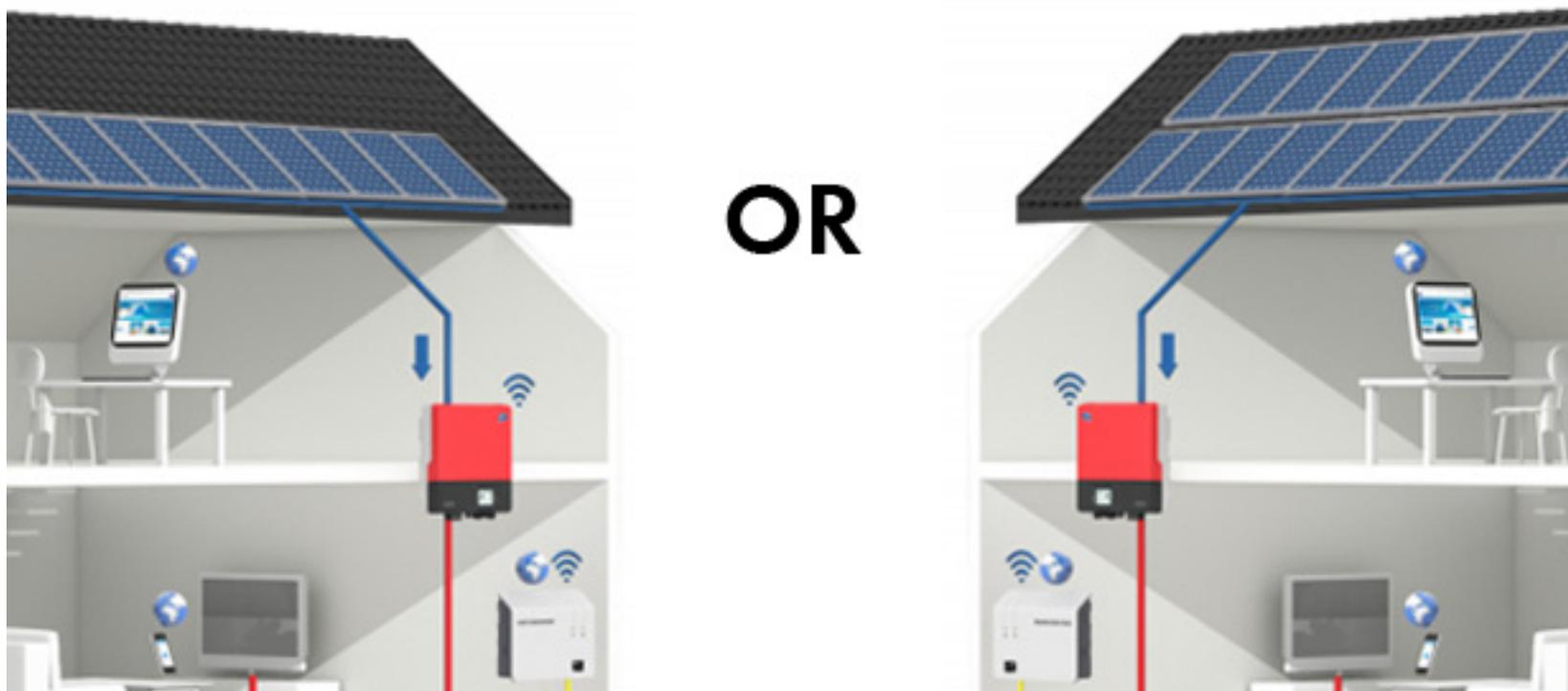
Oversizing a PV array, also referred to as undersizing a PV inverter, involves installing a PV array with a rated DC power (measured @ Standard Test Conditions) which is larger than an inverter's rated AC output power (i.e.  $DC @ STC > AC$ ). It can be a valuable tool for system designers seeking to deliver a maximum amount of energy at a lowest possible specific cost. Reasons for oversizing PV arrays and important factors to consider are summarised below.
