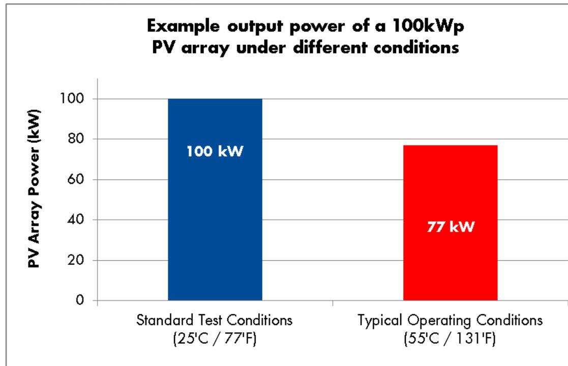
However it is obvious that a PV module would very rarely be subjected to these conditions under real world operating scenarios. Operating conditions can vary throughout the day and temperature can greatly impact the output power of a PV array. As the temperature of a PV array increases, its voltage and power will
