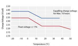
For continuous charging we recommend a voltage of  $2.25\,\mathrm{V}$  The charging voltage must be compensated to the curve for a continuously different battery ambient temperature
