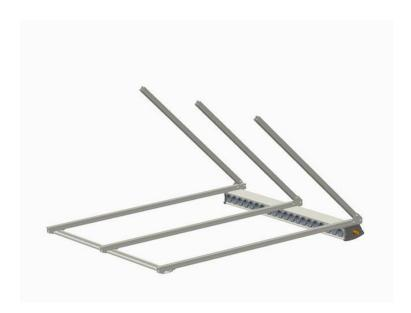
With the upper and lower manifolds and the three angled supports securely fastened, it is time to stand the semi-completed assembly onto its feet.
