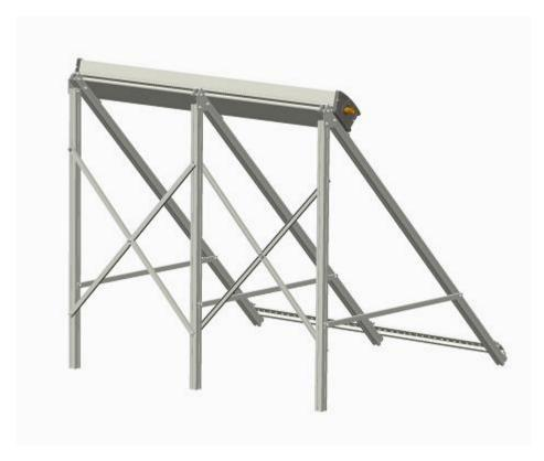
Fasten the four angled supports to the vertical up-rights of the pitching frame using the M8 x 25mm T-bolts and nuts provided. The supports are supplied with the pitching frame kit as are the stainless steel T-bolts and nuts. Note that the angled supports are also secured mid-length with a T-bolt and nut for extra support.
