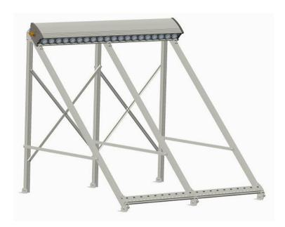
Finally, fasten the six pitching kit mounting feet to the vertical up-rights and angled manifold support system using the remaining M8 x 15mm T-bolts and nuts.
