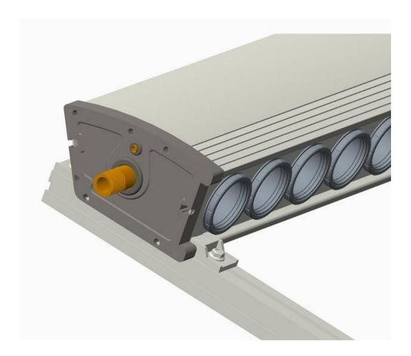
Fasten the ET upper manifold to the vertical supports using the Z-shaped brackets and fasteners included in the ET packaging. Ensure enough clearance is left to fasten both the top and the bottom of the manifold securely to the vertical supports (a total of six fasteners is provided).
