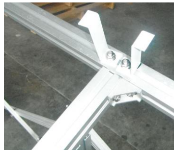
Fig 2. Top rail and 2 off 80mm panel supports (centre) fastened by T-bolts
